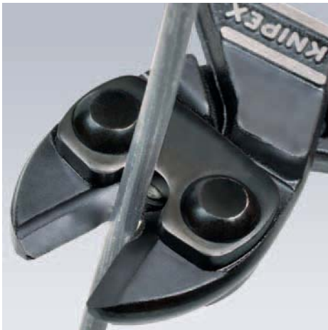
71 31/32/41 200: The cutting edge recess near the joint holds thicker wires in a favourable cutting position (optimum lever ratio). The re-positioning that is usual with bolt cutters is not needed here.
